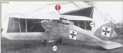
Rear view of the same aircraft shown above thought to be 5685/17. The top surface of the wings are covered with light 5 colour pre-printed lozenge fabric applied at a 45 degree angle. The cross fields seen here are noteworthy because this white square was superseded by a 5cm outline in November 1916. It is unlikely these were incorrectly applied at the Halberstadt factory and it is thought that some units backdated the newer markings either as a form of unit identification or to try and fool the enemy that they were flying in older, outdated equipment.
