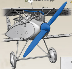
Nose detail from the unidentified early production Halberstadt Cl.II seen on page 25. Note the radiator pipe (F11), exhaust manifold, Niendorf propeller (94) and fat air pump of the 180hp Daimler-Mercedes D.IIIa engine.
