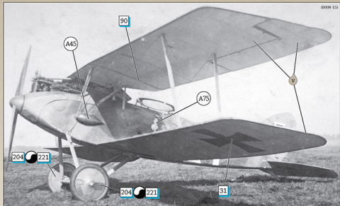
This early production Halberstadt Cl.II is thought to be 5717/17 from the first production order for 100 aircraft (numbers 5675/17 to 5774/17) placed in May 1917. Note the bulged generator fairing (A45) and 180hp Daimler-Mercedes D.IIIa engine.
