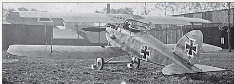
An unidentified early production Halberstadt Cl.II. Note the small rudder (F4), generator access cover (A45) and LMG 08/15 on the port side of the engine.
